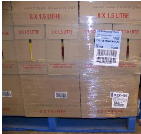
Figure 12: Example of the correct positioning of the pallet (logistics) Label
