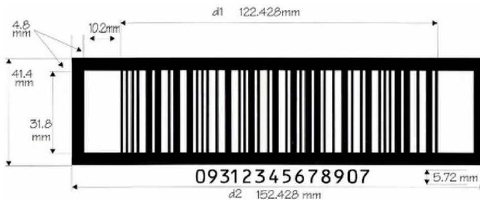
Figure 10: Nominal (100%) Magnified ITF-14 Barcode (not to scale)
