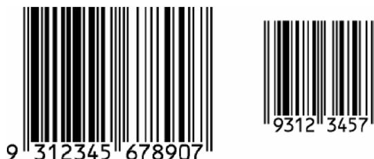
**Figure 2:** EAN-13 barcode & EAN-8 barcode
