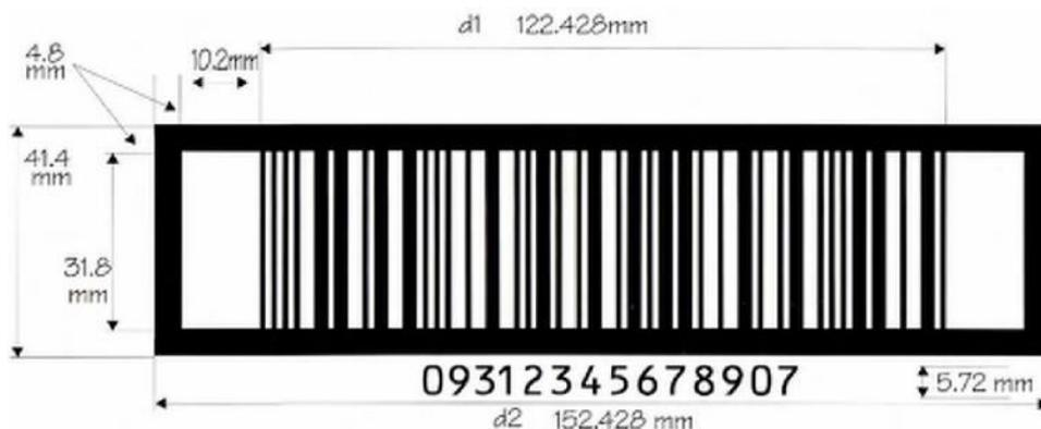
**Figure 10:** Nominal (100%) Magnified ITF-14 Barcode (not to scale)
