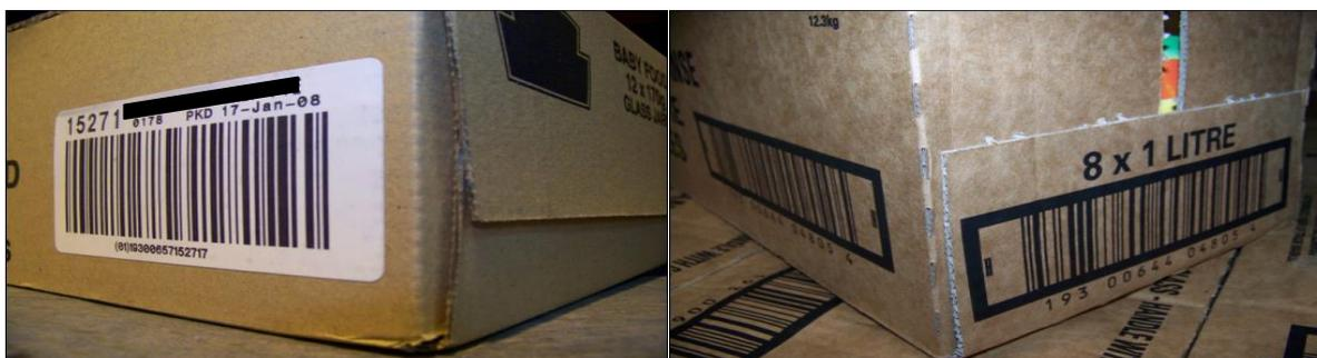
**Figure 8:** Barcode location on cartons – labels or pre-printed
